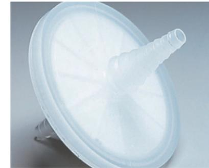
The CO<sub>2</sub> inlet is equipped with a high-efficiency microbial filter, with 99.99% filtration efficiency for particles larger than or equal to 0.2µm in diameter. It can effectively filter bacteria and dust particles in the CO<sub>2</sub> gas line to ensure the safety of experimental results.
